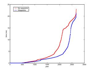
Figure 3: The effect of waypoints. The lines shows the sorted planning times for 2670 plans with and without waypoints, sorted by time to show the cumulative performance distribution. The upper (red) line shows performance without waypoints, while the lower (blue) line shows performance with waypoints (Waypoints=50, p[Waypoint]=0.4).
