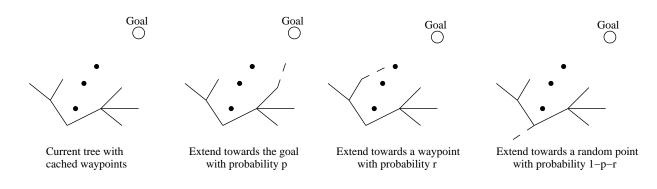
Figure 1: Extended RRT with a waypoint cache for efficient replanning.
