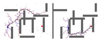
**Figure 2:** An example from the simulation-based RRT planner, shown at two times during a run. The tree grows from the initial state. The best plan is shown in bold, and cached waypoints are shown as small black dots.
